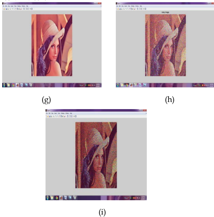
Fig.4.5: Results on LENA Image. (g) Original image (h) Noisy image with ND=30% (i) MDBUTMF
